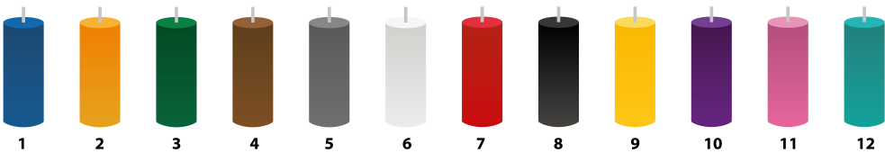
Colour coding (as per TIA-598-C)
