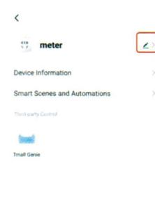
If equipment connect successfully , you can realize remote control on/off , timer control and delay time control , and read the energy and current /voltage/ active power and history energy data.
