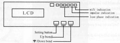
WiFi led indication, if you push the down button last 10s, the WIFI led will flash 1s interval ,its means meter enter into the status of waiting for WIFI distribution network . if WIFI led light on all time ,it means meter connect the WIFI successfully.
