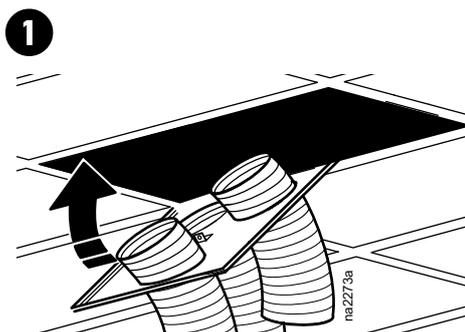
**NOTE:** Use 10-gauge (minimum) steel wire to support the ceiling tile adapter as shown. Ensure the wire is anchored to the building structural support (not the suspended ceiling frame).
