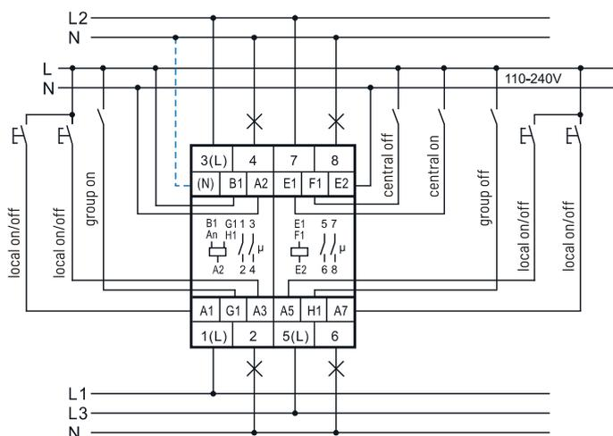
If N is connected, the zero passage switching is active at the contacts 1-2, 3-4 and 5-6.
